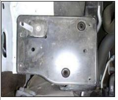
**4.** Remove the five 10mm bolts that secure the factory air filter housing platform and remove.
