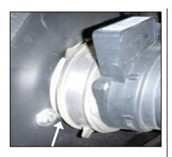
9. Slide the factory MAF meter into the black plastic filter adapter. Tighten hose clamp. (Note: The factory clamp / rubber bushing must be in place on the inlet to the MAF meter.) Reconnect the factory intake tube, and tighten clamp.
