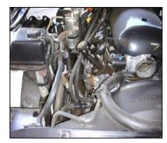
3. Remove the factory air filter lid and base from vehicle as an assembly. (Hint: pull straight up on the air filter base to remove, there are no bolts; just friction mounts).
