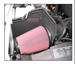
10. Mount the Airaid Premium Air Filter onto the black plastic filter adapter and tighten hose clamp. Press supplied weather stripping along the top edges of the Airaid cold air dam; assure that it is fully seated along the edges. (Hint: *Begin at a corner and work toward the ends*).
