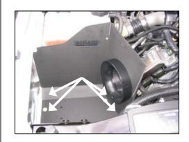
8. Position the Airaid Cool Air Dam Intake system in place of the factory air box & secure the Airaid system to the factory mounting pad using the four supplied 6mm bolts and washers. (Caution: over tightening may distort the cold air dam!)
