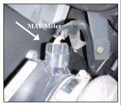
**2.** Unplug the MAF meter and remove the meter from the factory intake tube.
