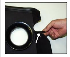
**6.** Install the 7 ¼" rubber trim onto the side of the air dam as illustrated.
