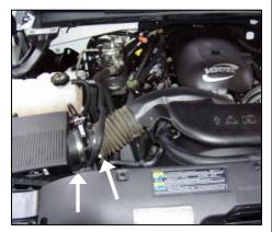
1. Disconnect the negative battery cable. Loosen the 2 factory hose clamps located at the Mass Air Flow (MAF) meter.
