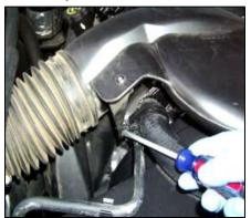
3. Using a flat head screwdriver, gently pry the radiator hose bracket from the factory intake tube assembly and remove from vehicle.
