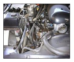
4. Remove the factory air filter, lid and base assembly & intake tube from vehicle. (Hint: pull straight up on the air filter base to remove, there are no bolts; just friction mounts).
