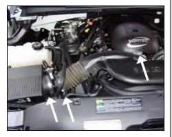
1. Disconnect negative battery cable. Loosen all three factory hose clamps located at the Mass Air Flow (MAF) meter and both ends of the factory intake tube.
