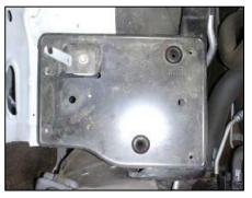
**5.** Remove the five 10mm bolts that secure the factory air filter housing platform and remove.
