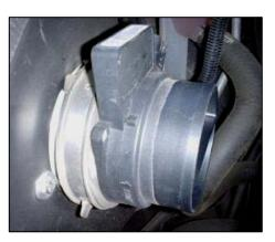
8. Slide the factory MAF meter onto the black plastic filter adapter. (*Note: factory clamp* / rubber bushing must be in place on the inlet to the MAF meter.)
