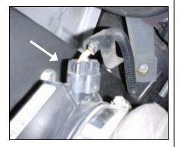
**11.** Reconnect the wiring harness to the MAF sensor.
