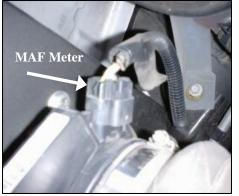
**2.** Unplug the MAF meter and remove the meter from the factory intake tube.
