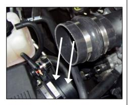
**10.** Install the hump hose provided onto the Airaid Intake Tube and the MAF with the supplied hose clamps. Install tube assembly onto engine. (*Hint: slide the hump hose all the way onto the end of the tube.*)
