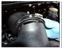
**9.** Install the GM coupler provided onto the throttle body side of the Airaid Intake Tube
