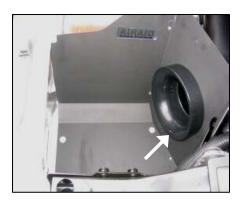
Install the black plastic filter adapter using the three ¼-20 x ½ button head bolts & three washers provided. Position the Airaid Cool Air Dam Intake system in place of the factory airbox & secure the Airaid system using the four supplied 6mm bolts and washers.
