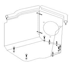
6. Position the two Airaid Cool Air Dam panels and fasten them together with the small #6 screws, nuts & washers provided.
