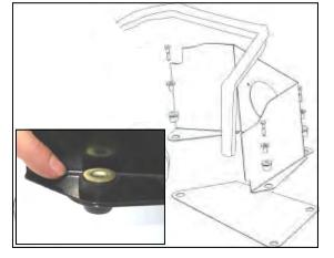
4. Assemble the Airaid Cool Air Dam panels (#2, #3) using the factory rubber grommets and inserts
