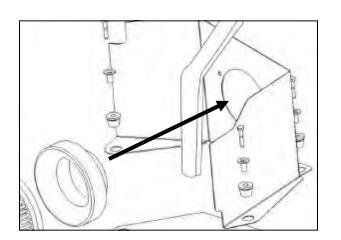
5. Install the filter adapter (#4) into the Airaid Cool Air Dam using three 1/4-20x 5/8" bolts (#6), and 1/4"
