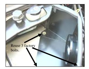
6. Install the Airaid Cool Air Dam over the three factory mounting points, and fasten with the
