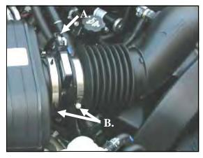
1. Disconnect the negative battery cable. A.) Disconnect the Mass Air Flow (MAF) sensor wiring harness. B.) Loosen the two hose clamps on the MAF sen-
