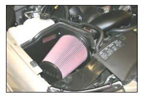
13. Install the Airaid Premium Filter (#1) onto the filter adapter (#5), and tighten the hose clamp. Next install the weather strip (#8) onto the top of the CAD as shown. For ease of installation start at the fender, and work towards the radiator.
