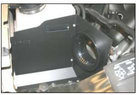
**9.** Install the assembled CAD in place of the factory airbox using four bolts (#11) and washers (#10). Do not over tighten the bolts.
