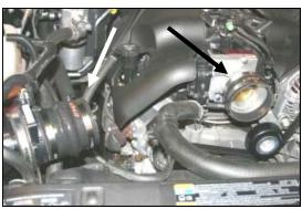
11. Install the hump hose (#6) on the Mass Air Flow sensor with two #56 hose clamps (#15). Next install the coupler (#7) on the throttle body with two #60 hose clamps (#16).
