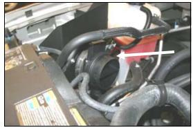
**10.** Re-install the Mass Air Flow sensor onto the filter adapter, and tighten the hose clamp. Make sure the rectangle area where the wiring harness connects is pointing straight up.
