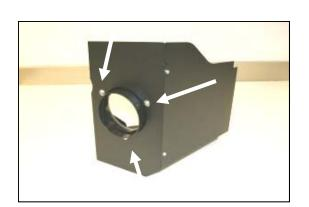
**8.** Install the filter adapter (#5) into the **CAD** using three button head bolts (#9), and washers (#10).
