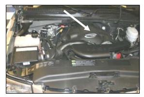
1. <u>Disconnect the negative battery cable.</u> With a 5/16" socket, remove one bolt on the top of the beauty cover. Set the bolt and the cover aside for re-installation later.
