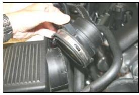
4. Without disconnecting the electrical connector, remove the Mass Air Flow sensor from the factory airbox, and set it aside.
