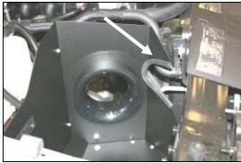
9. Install the assembled CAD in place of the factory airbox using four bolts (#11) and washers (#10). Do not over tighten the bolts. Install the rubber trim (#17) as shown at the arrow.
