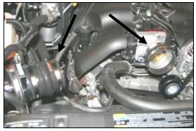
11. Install the hump hose (#6) on the Mass Air Flow sensor with two #56 hose clamps (#15). Next install the coupler (#7) on the throttle body with two #60 hose clamps (#16).
