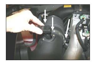
12. Re-position the factory intake tube onto the Airaid tube, and tighten the hose clamp. Next reinstall the Mass Air Flow sensor into the Airaid tube <u>using the two provided Button Head</u> <u>screws (#8)</u>. <u>Do not use the factory screws!</u> Do not over tighten!
