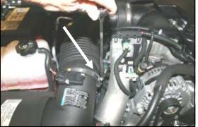
1. <u>Disconnect the negative battery cable.</u> With a 5/16" socket or flat screwdriver, loosen the hose clamp that holds the factory airbox to the flexible intake tube.
