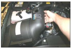
4. Slide the flexible intake tube off of the factory airbox and then rock the airbox back and forth to free it from the mounting grommets, then lift it straight up and remove it from the vehicle.
