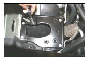
**6.** With a 10mm socket, remove 5 bolts from the factory airbox mounting plate. Remove the plate from the vehicle.
