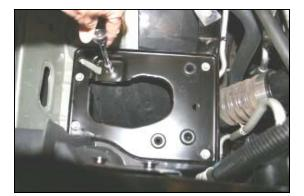
**6.** With a 10mm socket, remove 5 bolts from the factory airbox mounting plate. Remove the plate from the vehicle.
