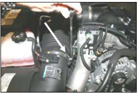
1. **Disconnect the negative battery cable.** With a 5/16" socket or flat screwdriver, loosen the hose clamp that holds the factory airbox to the flexible intake tube.
