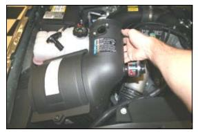
**4.** Slide the flexible intake tube off of the factory airbox and then rock the airbox back and forth to free it from the mounting grommets, then lift it straight up and remove it from the vehicle.
