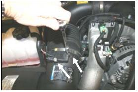
**2.** With a #20 Torx bit, remove 2 screws holding the Mass Air Flow sensor to the factory airbox tube.
