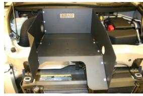
**6.** Assemble the three Cool Air Dam panels (#2, #3, & #4), using 13 screws (#11), washers (#12), and nuts (#13), as shown.
