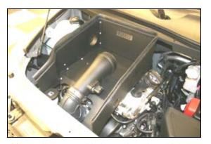
11. Install the assembled CAD into the vehicle by lowering the front into the vehicle first, and then aligning the two grommets on the studs at the rear of the engine. Push down firmly on the rear of the CAD to seat the grommets. Next slide the rubber elbow onto the Airaid Intake Tube.
