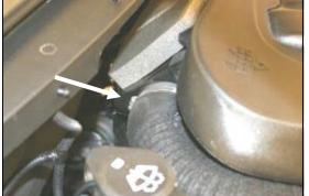
1. **Disconnect the negative battery cable.** With a 1/4" socket, loosen the hose clamp that holds the fresh air intake tube to the factory air cleaner housing. Slip the tube off of the factory air cleaner housing and set it aside, it will be reconnected later in the install.
