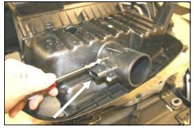
**4.** Using the supplied #20 torx bit, remove two screws, and the Mass Air Flow sensor from the factory air cleaner housing. Set it aside for reinstallation later in the install.
