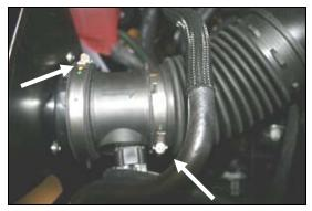
**9.** Re-install the Mass Air Sensor and coupler onto the air filter adapter (#4), as shown and tighten the hose clamp. Next re-connect the factory intake tube to the Mass Air Flow sensor, and tighten the hose clamp.
