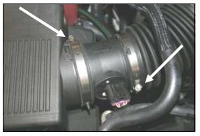
1. **Disconnect negative battery cable.** Loosen the hose clamp on the end of the factory intake tube at the Mass Air Flow sensor, next loosen the hose clamp that holds the Mass Air Flow sensor to the factory air box.
