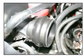
12. Install the hump hose (#6), and two #64 hose clamps (#16) onto the MAF sensor as shown. Tighten only the clamp on the MAF sensor at this time
