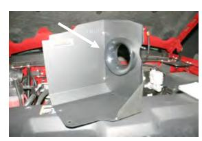
**9.** Assemble the Cool Air Dam panels (CAD) (#2 & #3) using five 3/16"screws (#10), washers (#11), and nuts (#12). Next install the filter adapter into the panels as shown using three 1/4" button head bolts (#13), and flat washers (#14).
