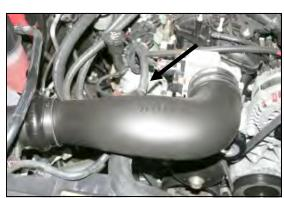
**14.** Install the Airaid Intake Tube into the hump hose first, and then onto the throttle body. Adjust it for fit, and tighten the hose clamps. Next install the 3/8" breather hose (#8) between the 3/8" barbed fitting in the tube, and the factory port on the valve cover.
