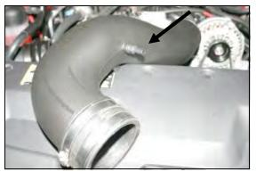
**13.** Install the 3/8" barbed fitting (#17) into the Airaid Intake Tube as shown. Next install the urethane coupler onto the throttlebody end of the tube using two #64 hose clamps (#16). Tighten *only* the clamp on the tube.
