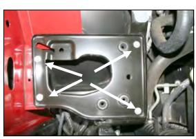
**8.** Using a 10mm socket, remove four bolts, and then remove the factory airbox mounting plate from the vehicle.
