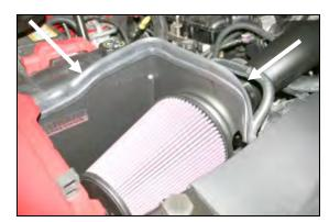
**15.** Install the Airaid Premium Filter (#1) onto the air filter adapter, and tighten the hose clamp. Next install the provided weather strip (#9) onto the top of the **CAD**. For ease of install, start at the inner fender, and work your way towards the radiator. Reinstall the beauty cover.
