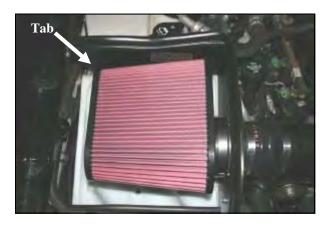
**13.** Install the Airaid Premium Filter (#1) onto the **MAF** sensor. Rotate the filter so that the tab contacts the air box base, and then tighten the clamp. Install the weather strip (#6) onto the top of the panel. (*Hint: Start at one end and work towards the other.*)
