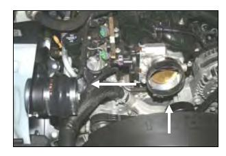
**9.** Slide the silicone hump hose (#4), and two #56 hose clamps (#14) onto the MAF sensor. Slide the coupler (#5) and one #68 hose clamp onto the throttle body. Tighten only the clamp on the **MAF** sensor for now.
