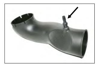
**10.** Insert one  $\frac{1}{4}$ " NPT x  $\frac{3}{8}$ " barbed fitting (#15) into the Airaid Intake Tube (#2).
