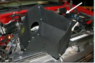
**2.** Assemble the three Cold Air Dam (CAD) panels (#s 2, 3, &4) as shown using nine 6-32 screws (#10), nine #6 washers (#9), and nine nuts (#11).
