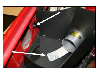
**6.** Install the **CAD**/Tube assembly into the vehicle as shown using two 5/16"x 1" bolts (#13) thru the 3" x 2" plate (#12) up thru the fender well, thru the **CAD**, and thru the bracket on the intake tube, secured with two 5/16" flat washers (#14) and two 5/16" nylock nuts (#15). Next secure the **CAD** to the side fender well using one 1/4" hex bolt (#16), 1/4" flat washer (#8), and 1/4" serrated nut (#17). Refer to the line drawing above if needed.
