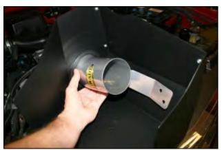
**4.** Insert the Airaid intake tube (#5) thru the hole in the **MAF** panel and then rotate it clockwise so that the holes in the bracket on the tube line up with the two holes in the bottom panel.
