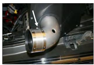
**5.** Install the stainless steel coupler (#6) onto the Airaid intake tube and tighten *only* the hose clamp on the tube.
