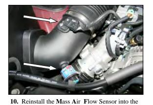
Airaid Intake Tube using the supplied 8-32x1/2" button head screws (#8).
