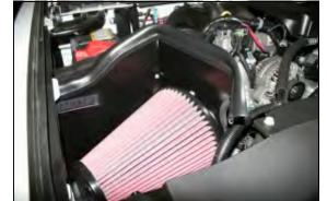
11. Install the Airaid Premium Filter (#1) onto the Airaid intake tube (#4), and tighten the hose clamp. Now install the provided weather strip (#5) on the top of the CAD. For ease of installation, start near the fender and work your way towards the radiator.
