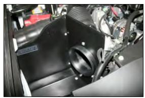
**8.** Install the Cool Air Dam into the vehicle where you removed the factory mounting plate in step #4, using the four supplied M6-1x25 bolts (#9), and flat washers (#7). **Do Not Over Tighten** the Bolts!
