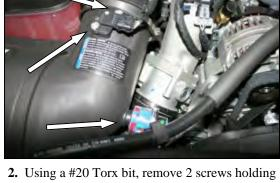
the Mass Air Flow sensor to the factory airbox tube. Remove the MAF and set it aside. Remove the factory filter minder and grommet from the factory airbox. Save them for later use in step #10.
