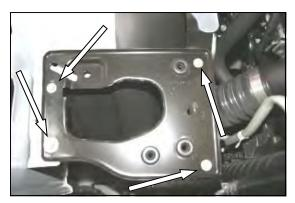
**4.** Using a 10mm socket, remove 4 bolts from the factory airbox mounting plate. Remove the plate from the vehicle.
