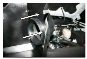
7. Install the supplied rubber trim (#13) onto the Cool Air Dam as shown.
