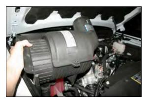
**3.** Slide the flexible intake tube off of the factory airbox and then rock the airbox back and forth to free it from the mounting grommets, next lift it straight up and remove it from the vehicle.
