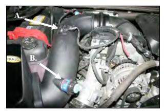
**7. A.)** Reinstall the Mass Air Flow sensor into the Airaid Intake Tube using two 8-32x 3/8" button head screws (#8). **Do Not Use The Factory Screws!** It may be necessary to reroute the MAF sensor wiring harness so that it will reach the proper location in the tube.
