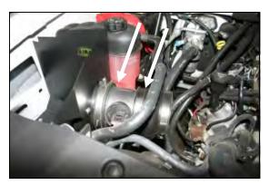
**10.** Reinstall the **MAF** sensor onto the filter adapter, and tighten the clamp. Next install the urethane hump hose (#6) onto the **MAF** with the two #64 hose clamps (#16). Tighten only the hose clamp that secures it to the **MAF**.
