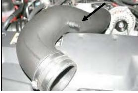
**11.** Install the 1/4" NPT x 3/8" Barb Fitting (#18) into the Airaid Intake Tube as shown. Next install the urethane coupler (#7) onto the throttle body end of the tube using two #64 hose clamps (#17). Tighten *only* the clamp on the tube.
