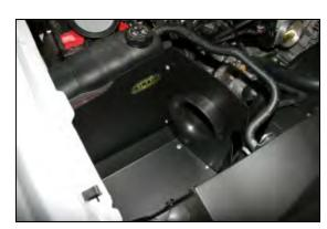
**9.** Install the Airaid **CAD** assembly into the vehicle replacing the factory airbox. Secure the **CAD** using four M6 x 1.25 Hex Bolt (#16), and 1/4" flat washers (#15). Do not over tighten the four bolts.
