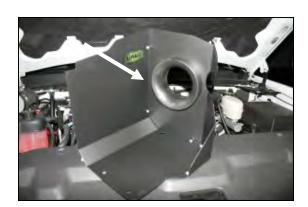
**8.** Assemble the Cool Air Dam panels (CAD) (#2 & #3) using five 6-32 x 5/16" screws (#10), #6 flat washers (#11), and 6-32 keps nuts (#12). Next install the air filter adapter (#5) into the panels as shown with the hole for the Mass Air Flow sensor facing up, using three 1/4 - 20 x 1/2" button head bolts (#14), and 1/4" flat washers (#15).
