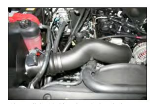
**12.** Install the Airaid Intake Tube into the hump hose first, and then onto the throttle body. Adjust it for fit, and then tighten all three hose clamps. Reinstall the plastic retainer on the radiator hose into the bottom of the Airaid Intake Tube. Refer to step #3.
