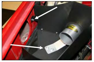
**7.** Install the **CAD**/Tube assembly into the vehicle as shown using two supplied 5/16"x 1" bolts (#10) thru the 3" x 2" plate (saved from step #2 ) up thru the fender well, thru the **CAD**, and thru the bracket on the intake tube, secured with two supplied 5/16" flat washers (#11) and two 5/16" nylock nuts (#12). Next secure the **CAD** to the side fender well using one 1/4" hex bolt (#13), 1/4" flat washer (#6), and 1/4" serrated nut (#14). Refer to the line drawing above if needed.
