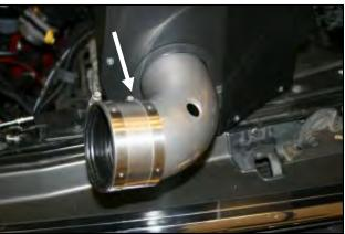
4. Install the supplied rubber trim (#15) into the hole in the MAF Panel (#2) as shown.
