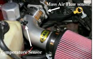
1. Disconnect the negative battery cable. VERY CAREFULLY! Remove the air intake temperature sensor first, and then the grommet from the air intake tube and set them aside. There is no need to disconnect the wiring harness on the temp sensor. Loosen the two hose clamps on the stainless steel cou-
