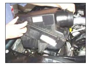
**3.** Remove the factory intake tube assembly from the engine. Rock the factory air box back and forth and remove it from it's mounting. There are only grommets holding it in, no bolts.
