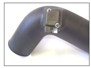
**9.** Using two 8-32 x 1/2" button head screws (#10) install the factory **M.A.F.** sensor in the Airaid intake tube (#2) **DO NOT USE THE FACTORY SCREWS!**
