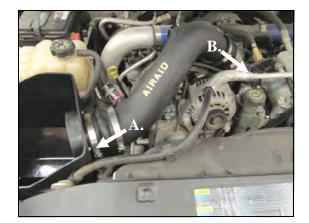
13. A.) Install the hump hose end of the Airaid intake tube assembly onto the filter adapter first.B.) Slip the coupler end of the tube over the factory turbocharger inlet. Adjust for fit, and tighten the hose clamps
