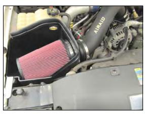
**14.** Install the Airaid Premium Filter (#1) onto the filter Adapter, and tighten the hose clamp. Install the Weather Strip (#7) onto the Airaid Cold Air Box. Reconnect the **M.A.F.** sensor wiring harness. (*Note: Start from one corner and work your way around to insure proper alignment of the weather strip.)*
