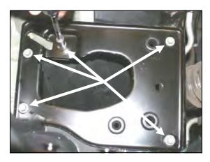
**4.** Using a 10mm socket, remove the five bolts and mounting plate from the engine compartment and set aside. Three of these bolts will be re used in step 6.
