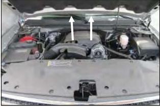
1. <u>Disconnect the negative battery cable.</u> Remove the engine cover by simply pulling up on it and sliding out from the vehicle.
