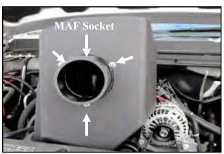
**8.** Install the Filter Adapter (#4) onto the Cold **Air Box** or **CAB** (#3) as shown using the three 1/4-20 Button Head Screws (#10) and 1/4" Flat Washers (#11). Note: The MAF socket is to be in the 12:00 position when properly assembled.
