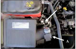
Disconnect the Mass Air Flow or MAF sensor (A) and the Manifold Absolute Pressure or MAP sensor (B) Remove the factory airbox from the vehicle.
