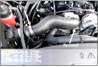
**11.** Install the Airaid Intake Tube assembly onto the Filter Adapter first, and then onto the throttlebody. Adjust for fit, and tighten all hose clamps. Reinstall the hose anchor into the Airaid Intake Tube.
