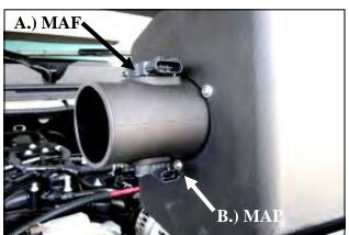
**8.** Install the Filter Adapter (#4) onto the Cold Air Box or CAB (#3) as shown using the three 1/4-20 Button Head Screws (#10) and 1/4" Flat Washers (#12). **A.**) Transfer the MAF sensor from the factory airbox into the Filter Adapter. Secure the sensor using the two 8-32 Button Head Screws (#9).
