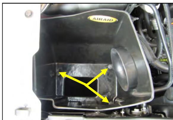
**5.** Slide the Airbox assembly into the inner fender area and secure it using 3 of the OEM bolts removed in step 3.
