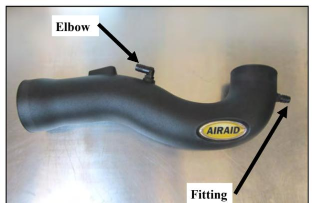
**6.** Install the Barbed Fitting and Elbow (#s 13 and 14) into the Airaid Intake Tube as shown.
