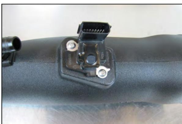
**7.** Transfer the Mass Air Flow sensor from the factory airbox into the Airaid Intake Tube. Secure the sensor using the two 8-32 Button Head Screws (#17).
