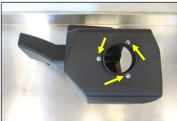
**4.** Install the Filter Adapter onto the Cold Air Box as shown using the three 1/4-20 Button Head Screws (#15) and 1/4" Flat Washers (#16).
