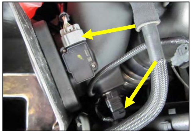
16. Reconnect the Mass Air Flow sensors. Note: the Extension Harness is to be routed underneath the Intake Tube.
