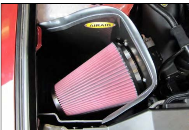
17. Install the Airaid Premium Filter onto the Intake Tube inside of the Cold Air Box. Install the Weather Strip onto the top edge of the Cold Air Box with the contour rolling away from the filter.
