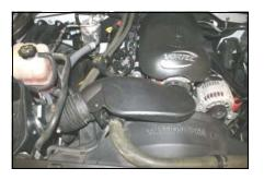
**10.** Re-install the intake tube and tighten the hose clamps. Re-install the plastic holder from step #1.
