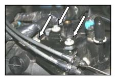
**8.** Re-install the throttle cable bracket and the 3 factory bolts removed in step 4. Some minor adjustments to the extension plates may be necessary to get all three bolts to be aligned in position.
