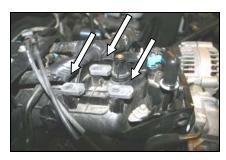
**5.** Install three 1/2" extension plates (#3) using the provided flat head countersunk bolts(#4). Point the long end towards the radiator, and snug them down.
