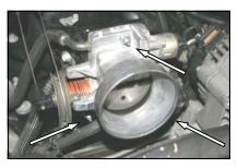
**2.** With a 10mm socket, remove the three nuts that hold the throttle body to the intake manifold.
