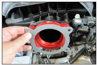
**3.** Install the Poweraid Spacer into the intake manifold with the supplied gasket on the throttlebody side, as shown. Make sure the "flow" arrow that is printed on the spacer is pointing towards the intake manifold.
