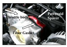
5. Install 2 of the supplied bolts (#2) and washers (#3) thru the two holes in the top of the throttle body, thru the supplied fiber gasket (#4), thru the Poweraid Spacer, and into the two brass inserts in the intake manifold. Run the bolts in a few threads with your fingers. Use caution not to cross-thread the bolts. Next install the 2 remaining bolts (#2) and washers (#3) in the two bottom holes of the throttle body, and tighten in a cross pattern to the vehicle manufacture's specifications.
