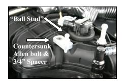
**6.** Remove the "ball stud" from the top of the intake manifold, insert the countersunk Allen bolt (#6) thru the countersunk hole in the provided 3/4" spacer plate (#5). Thread the countersunk bolt into the hole where you removed the "ball stud", face the spacer towards the front of the vehicle, and tighten the countersunk Allen bolt. Next thread the "ball stud" into the forward hole in the 3/4" spacer and tighten.
