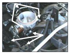
**3.** With a 10mm deep well socket, remove the throttle body, throttle cable support bracket, and throttle cable bracket nuts. Using a 6mm 12 point socket, remove the rear stud from the throttle body. Disconnect the harness plugs on the throttle body.
