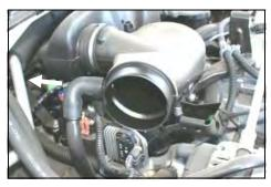
**2.** Disconnect the breather hose elbow from the intake hat. Remove the intake hat, and hold down nut, and save them for reuse.
