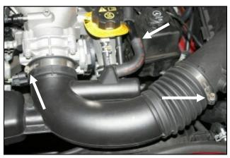
2. Disconnect the breather hose elbow at the hard plastic breather tube. Loosen the two hose clamps that secure the intake tube to the throttlebody, and the air cleaner lid.
