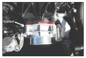
**5.** Vehicles equipped with plastic intake manifolds have an O ring pressed into the throttle body mounting surface. On these applications only a single gasket is to be used between the spacer and the throttle body. Discard the second gasket.
