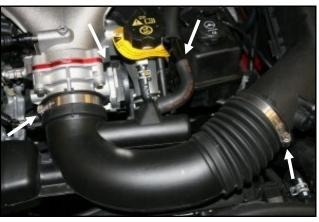
**6.** Reinstall the intake tube, tighten the two hose clamps, and reconnect the crankcase breather tube. Reinstall the beauty cover, and oil cap in the reverse order that they were removed. **Re-connect the negative battery cable!**
