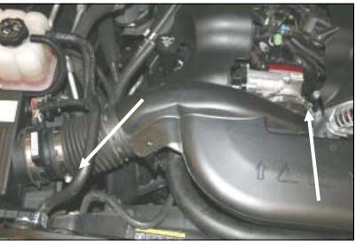
**2.** Loosen the hose clamps on both ends of the factory intake tube.
