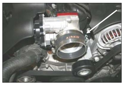
**5.** Install the coupler (#4) and two #60 hose clamps (#6) on the throttle body as shown. Leave the hose clamps loose for now.
