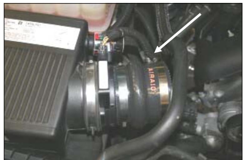
**4.** Install the hump hose (#3) and two #56 hose clamps (#5) on the Mass Air Flow sensor as shown. Leave the clamps loose for now.
