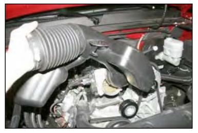
5. Slide the factory intake tube off of the MAF sensor, rotate it up so that it disengages from the mounting grommet on the intake manifold, and then slide it forward off of the throttle body and remove it from the vehicle.
