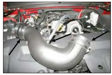
6. Install the silicone coupler (#4) on the throttle body end of the Modular Intake Tube (#2) with two #60 hose clamps (#6). Install the urethane hump hose (#3) on the other end of the MIT with two #64 hose clamps (#7). Leave all clamps loose for now. Install the 3/8" barbed fitting (#8) into the MIT, and slide the 3/8" breather hose (#5) over the barbed fitting as shown.
