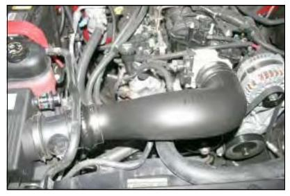
**9.** Install the **MIT** onto the **MAF** first, and then onto the throttle body. Adjust for fit, and tighten the hose clamps. Next connect the breather hose to the factory breather port on the valve cover. Reinstall the factory hose clamp barb back into the hole in the bottom of the **MIT**. Reinstall the beauty cover.
