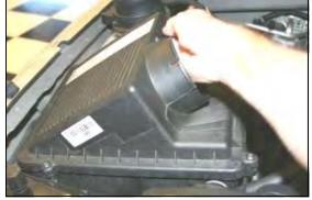
**4.** Grab the factory airbox and rock it back and forth, and remove it from the vehicle. It is only held in by grommets, no bolts.
