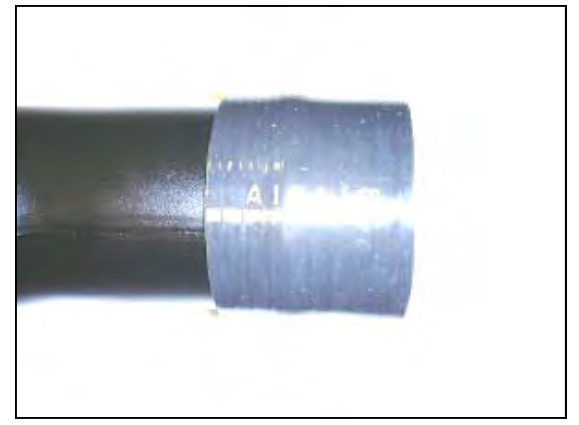
12. Install the urethane coupler (#7) and two #60 hose clamps (#18) onto the small end of the Airaid intake tube. (Note: Leave hose clamps loose until final assembly.)
