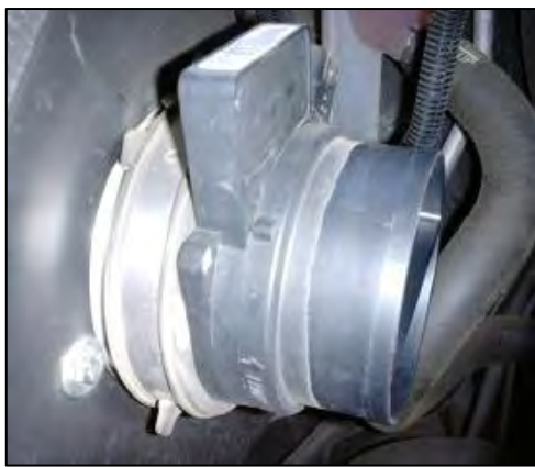
10. Install the MAF sensor to the filter adapter (#4), and tighten the hose clamp .
