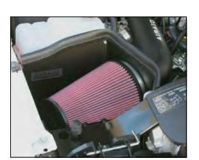
**13.** Install the Airaid filter (#1) onto the filter adapter, and tighten the hose clamp. Install the weather strip (#8) onto the Airaid Cool Air Dam. Reconnect the **MAF** sensor wiring harness. (*Note: Start from one corner and work your way around to insure proper alignment of the weather strip.)*
