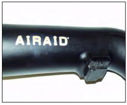
**8.** Using two 8-32x 1/2" button head screws (#15) install the factory **M.A.F.** sensor in the Airaid intake tube (#5) **DO NOT USE THE FACTORY SCREWS!.** (*Note: Sensor must be installed in the direction shown in the picture.*)
