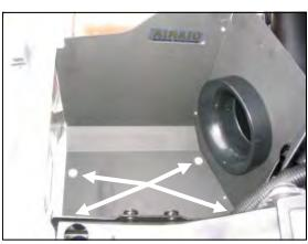
**7.** Install the Airaid Cool Air Dam assembly in the engine compartment using four M6-1x25 hex bolts (#14) and 1/4" flat washers (#13).
