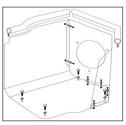
**5.** Assemble the Airaid Cool Air Dam panels (#2, #3) using five 6-32 x 5/16" screws (#9), #6 flat washers (#10) and 6/32 keps nuts (#11).
