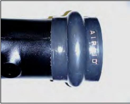
**10.** Install the urethane hump hose (#6) and two #72 hose clamps (#16) onto the large end of the Airaid intake tube. (*Note: Leave hose clamps loose until final assembly.*)
