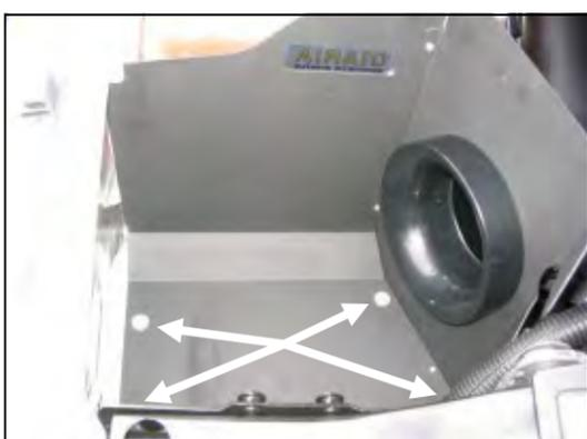
**7. Install the Airaid Cool Air Dam assembly in the engine compartment using four M6-1x25 hex bolts (#14) and 1/4" flat washers (#13).**
