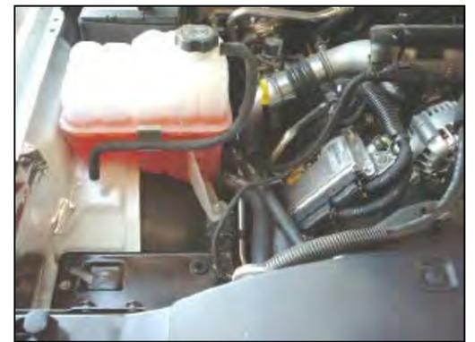
**3. Remove the factory intake tube assembly** from the engine. Rock the factory air box back and forth and remove it from the vehicle. There are only grommets holding it in, no bolts.
