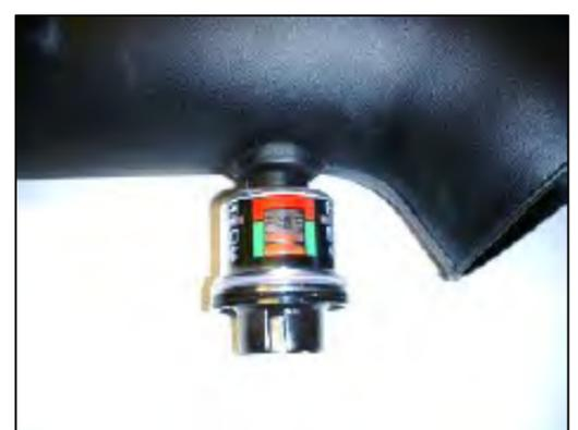
**9. Install the factory rubber grommet and air filter minder into the Airaid intake tube.**
