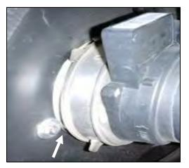
9. Slide the factory MAF meter onto the filter adapter. Tighten the hose clamp. (Note: The factory clamp / rubber bushing must be in place on the inlet to the **MAF** meter.) Reconnect the factory intake tube, MAF meter wiring harness, and tighten the clamps.
