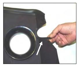
**6.** Install the  $7\frac{1}{4}$ " rubber trim (#12) onto the side of the Airaid Cool Air Dam.
