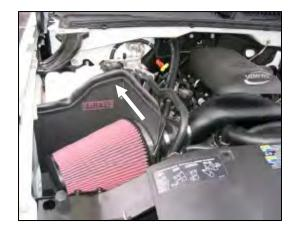
**12.** Press the weather strip (#8) along the top edges of the Airaid Cool Air Dam; assure that it is fully seated along the edges. (Hint: *Begin at a corner and work toward the ends*). Mount the Airaid Premium Filter (#1) onto the air filter adapter and tighten the hose clamp.
