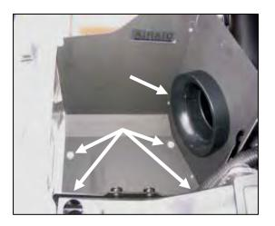
**7.** Install the air filter adapter (#4) using three  $\frac{1}{4}$ -20x  $\frac{1}{2}$ " button head bolts (#12), and  $\frac{1}{4}$ " flat washers (#13). Position the Airaid Cool Air Dam in place of the factory airbox & secure it with four M6-1x25 hex bolts (#14) and  $\frac{1}{4}$ " flat washers (#13).
