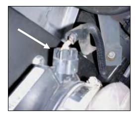
**11.** Reconnect the wiring harness to the **MAF** sensor.
