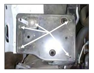
**5.** Using a 10mm socket, remove the five bolts that secure the factory air filter housing platform and
