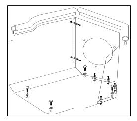
**6.** Assemble the Airaid Cool Air Dam panels (#2, #3) using five 6-32x 5/16" screws
