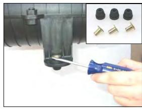
**3.** Remove the factory airbox and set it aside. Using a flat blade screwdriver, remove and save the three factory rubber grommets and inserts from the airbox base.
