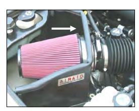
**8**. Install the Airaid Premium Filter (#1) onto the filter adapter, and tighten the hose clamp. Install the provided weather strip (#5) onto the top edge of the panel. (Hint: Start at one end, and work to the other.)
