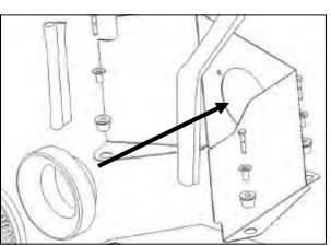
6. Install the Airaid Cool Air Dam over the three factory mounting points, and fasten with the factory bolts saved in step #2.
