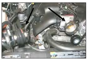
**11.** Install the urethane hump hose (#6) on the **M**ass **Air F**low sensor with two #60 hose clamps (#15). Next install the urethane coupler (#7) on the throttle body with two #64 hose clamps (#16).
