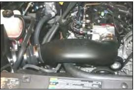
**12.** Install the Modular Intake Tube into the hump hose first, and then into the throttle body. Adjust for fit, and tighten all four hose clamps. Re-insert the plastic piece from step #3 into the hole on the bottom of the **MIT**.
