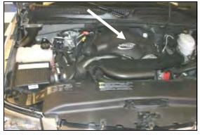
1. **Disconnect the negative battery cable.** Using a 5/16" socket, remove one bolt on the top of the beauty cover. Set the bolt and the cover aside for re-installation later.
