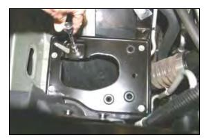
**6.** Using a 10mm socket, remove 5 bolts from the factory airbox mounting plate. Remove the plate from the vehicle.
