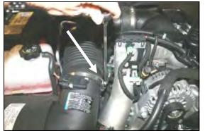
1. **Disconnect the negative battery cable.** Using a 5/16" socket or flat screwdriver, loosen the hose clamp that holds the factory airbox to the flexible intake tube.
