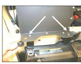
**8.** Install the two large factory grommets removed from the factory air cleaner housing in step #5, into the two holes at the back of the Airaid Cool Air
