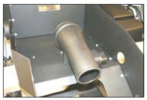
**10.** Install the Airaid Intake Tube onto the **CAD** using two 1/4-20 x 1/2" button head bolts (#7) and 1/4" flat washers (#8), threaded up from the bettom of the **CAD**.
