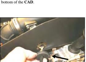
**13.** Slide the Mass Air Flow sensor connector thru the hole in the side of the **CAD**, and install the "split" grommet (#16) over the wiring loom as shown.
