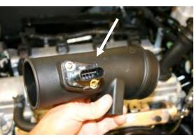
9. Install the Mass Air Flow sensor removed in step #4, into the Airaid Intake Tube (#5) using the two 8/32"x 3/8" button head screws (#10).
