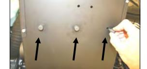
7. Install the three silicone bumpers (#15) into the three holes in the bottom of the Cool Air Dam, as shown.
