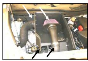
**15.** Install the Airaid Premium Filter (#1) onto the Airaid Intake Tube, and tighten the clamp. Install the weather strip (#6) on top of the **CAD** starting at the front corner, and working your way to the other corner. Reconnect the factory fresh air tube to the **CAD**, and tighten the hose clamp. Adjust the factory rubber elbow on the Airaid Intake Tube, and tighten the hose clamp.
