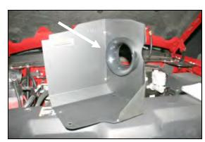
9. Assemble the Cool Air Dam panels (CAD) (#2 & #3) using five 6-32 x 5/16" screws (#10), #6 flat washers (#11), and 6-32 keps nuts (#12). Next install the air filter adapter (#5) into the panels as shown using three 1/4 -  $20 \times 1/2$ " button head bolts (#13), and 1/4" flat washers (#14).
