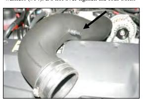
**13.** Install the 1/4" NPT x 3/8" Barb Fitting (#17) into the Airaid Intake Tube as shown. Next install the urethane coupler (#7) onto the throttle body end of the tube using two #64 hose clamps (#16). Tighten *only* the clamp on the tube.
