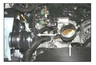
**9.** Slide the silicone hump hose (#4), and two #56 hose clamps (#14) onto the MAF sensor. Slide the coupler (#5) and one #68 hose clamp onto the throttle body. Tighten only the clamp on the **MAF** sensor for now.
