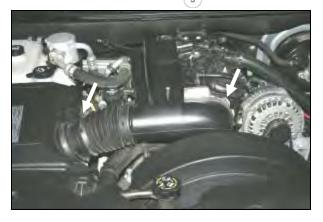
**2.** Using a 5/16" socket or flat blade screwdriver, loosen the hose clamps on both ends of the factory intake tube.
