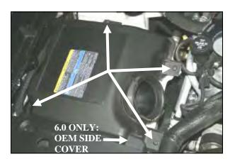
**5.** <u>6.0 Liter Only:</u> Using a flat blade screwdriver, gently pry the plastic retaining clip from the oem side cover.
