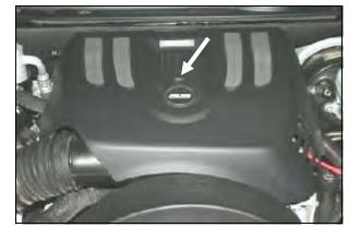
**1.** <u>Disconnect the negative battery cable.</u> <u>6.0 Liter Only:</u> Using a T-30 torx bit, remove the factory screw and engine beauty cover, and then set them aside for reuse.
