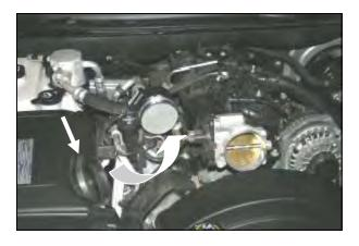
**4.** Loosen the clamp holding the Mass Air Flow (MAF) sensor to the factory airbox lid. Remove the complete factory intake and breather tube. Remove
