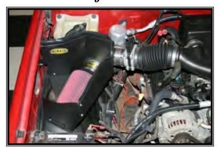
Synthamax Air Filters <u>do not</u> require <u>oil</u>. Service air filter as needed by cleaning with common non-petroleum all-purpose household cleaner and water. Simple Green®, Formula 409® or equivalent works great. Apply cleaner to outside of air filter and allow to soak. Then flush filter clean from the inside out with a garden hose and repeat steps if necessary. Do not apply high pressure water or air to clean filter. Allow filter to air dry and reinstall.
