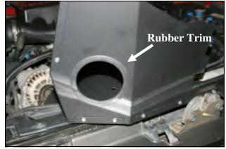
**3.** Install the supplied rubber trim (#18) into the hole in the **MAF** Panel (#2) as shown.
