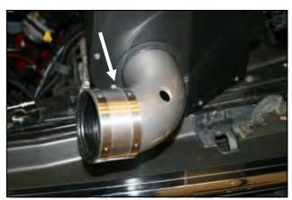
**5.** Install the stainless steel coupler (#6) onto the Airaid intake tube and tighten *only* the hose clamp on the tube.
