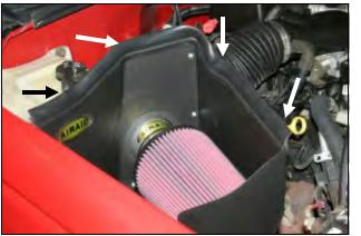
**8.** Install the Airaid Premium Filter (#1) onto the Airaid intake tube as shown, and then tighten the hose clamp. Next, install the weather strip on top of the **CAD**, starting at the right fender working your way towards the front of the vehicle.
