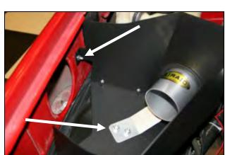
**6.** Install the **CAD**/Tube assembly into the vehicle as shown using two 5/16"x 1" bolts (#13) thru the 3" x 2" plate (#12) up thru the fender well, thru the **CAD**, and thru the bracket on the intake tube, secured with two 5/16" flat washers (#14) and two 5/16" nylock nuts (#15). Next secure the **CAD** to the side fender well using one 1/4" hex bolt (#16), 1/4" flat washer (#8), and 1/4" serrated nut (#17). Refer to the line drawing above if needed.
