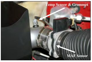
**7.** Connect the **MAF** sensor to the stainless steel coupler and tighten the hose clamp. Install the factory grommet removed in step #1, into the hole in the Airaid intake tube. **VERY CAREFULLY** install the factory temperature sensor into the grommet.
