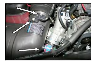
2. Using a #20 Torx bit, remove 2 screws holding the Mass Air Flow sensor to the factory airbox tube. Remove the MAF and set it aside. Remove the factory filter minder and grommet from the factory airbox. Save them for later use in step #10.
