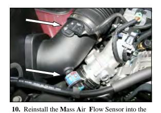
Airaid Intake Tube using the supplied 8-32x1/2" button head screws (#8). **Do Not Use The Factory Screws!**
