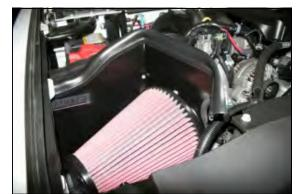
11. Install the Airaid Premium Filter (#1) onto the Airaid intake tube (#4), and tighten the hose clamp. Now install the provided weather strip (#5) on the top of the CAD. For ease of installation, start near the fender and work your way towards the radiator
