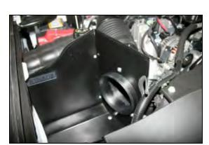
**8.** Install the Cool Air Dam into the vehicle where you removed the factory mounting plate in step #4, using the four supplied M6-1x25 bolts (#9), and flat washers (#7). **Do Not Over Tighten** the Bolts!
