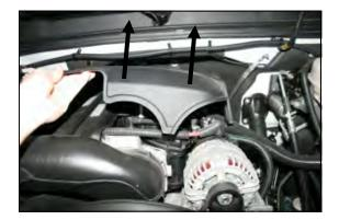
**1.** Disconnect the negative battery cable. Remove the factory beauty cover by lifting up on the front, and then pulling the cover towards the front of the vehicle. It is only held in place by grommets.
