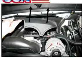
1. Disconnect the negative battery cable. Remove the factory beauty cover by lifting up on the front, and then pulling the cover towards the front of the vehicle. It is only held in place by grommets.
