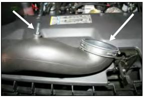
**11.** Install the 1/4" NPT x 3/8" Barb Fitting (#18) into the Airaid Intake Tube as shown. Next install the supplied coupler and hose clamp (#7) onto the throttle body end of the tube. Leave the clamp loose for now.
