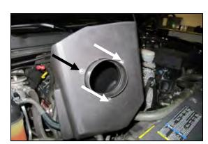
**9.** Install the Filter Adapter (#4) onto the Cold Air **B**ox, or **CAB** (#3), as shown using the three 1/4-20 Button Head Bolts (#9) and 1/4" Washers (#10).
