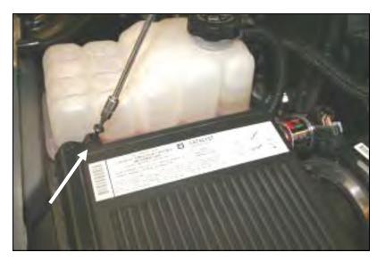
**8.** If you purchased the 201-719 Jr. Kit, remove 4 screws in the factory airbox with a #25 Torx bit, and remove the factory air filter.
