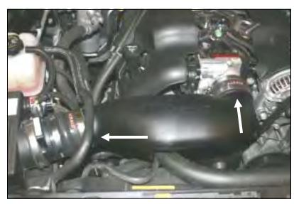
**6.** Install the Modular Intake Tube (#2) into the hump hose first, and then into the throttle body. Adjust for fit, and tighten all four hose clamps. Re-insert the plastic piece from step #3 into the hole on the bottom of the MIT.
