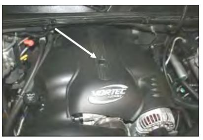
1. <u>Disconnect negative battery cable.</u> With a 5/16" socket, remove one bolt on the top of the beauty cover. Set the bolt and the cover aside for reinstallation later.
